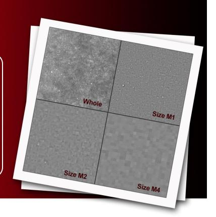
The OMA uses a wavelet-based technique that partitions print/coating mottle into its size components.
