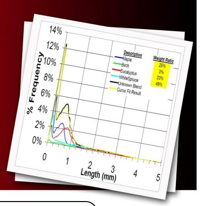
Fiber morphological data of 100% Pure pulp samples, collected by either the FQA-360 or the HiRes FQA, is used in combination with the fiber morphological data of blends with known mass ratio, to estimate the mass ratio of an unknown blend. Up to 5 species components may be estimated to an accuracy approaching 1% by weight.
