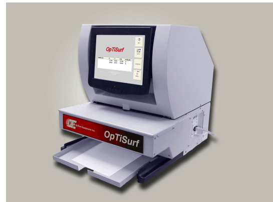
OpTiSurf measures optically the surface roughness of sheets
